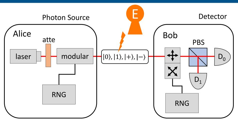
RNG: random number generator PBS: polarizing beamsplitter atte: attenuator
